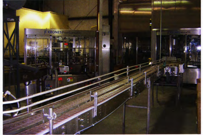
FIGURE 1.3. The location and orientation of packaging machinery is often specified to accommodate constraints in existing building space. (Courtesy Trumer Brauerei-Berkeley)
