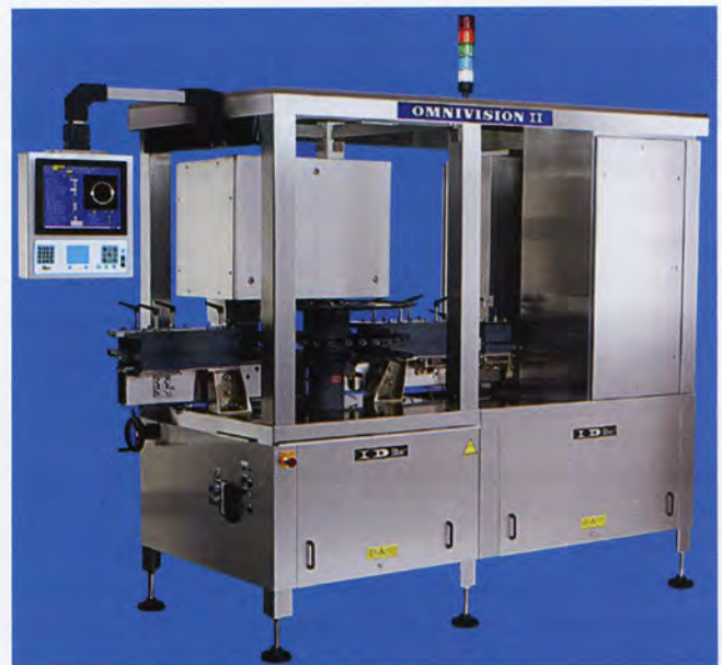
FIGURE 1.1. An electronic bottle inspector on a brewery bottling line performing base and neck finish inspection; the soft-push ram and chute are at the right. (Courtesy Industrial Dynamics Company)
